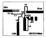
Material: Epoxy; size 24mm x 30mm; thickness 1mm
