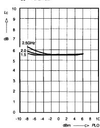
Conversion Loss Lc = f(VDD) PLO = 0dBm $f_LO = 1500MHz$ ;  $f_IF = 120MHz$
