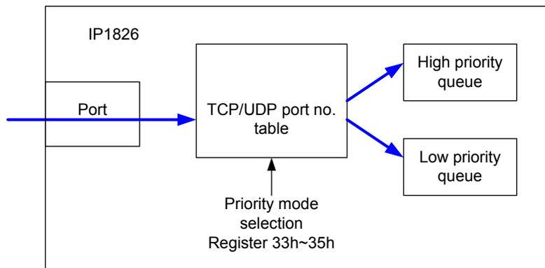
A packet with TCP/UDP port number defined as low priority in register 33h~35h will be treated as a low priority packet if register 01h[8] is set to “1”; regardless port based/ tag based/ IP based priority setting. That is, it overwrites other settings.
